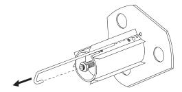
**11.** If you are using a core, slide it onto the rewind spindle until it is flush against the guide plate.
